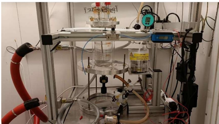
Figure 1: Small pilot scale setup for continuous electrochemical lignin depolymerization.
