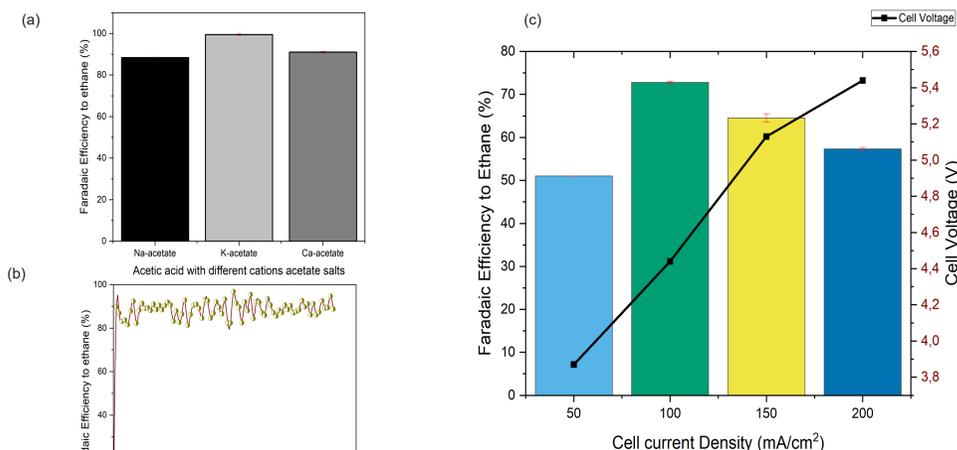
Figure 4. Faradaic efficiency to Kolbe product ethane (a) Impact of cations from supporting electrolyte toward F.E. (averaged) to ethane at pH 5 and 25mA/cm<sup>2</sup> on platinum foil in three electrode batch cell. (b) Continuous monitoring of F.E. for 6.5 hours in 1M Na-acetate at pH 5 and 25mA/cm<sup>2</sup> (c) Kolbe electrolysis of Na-acetate and acetic acid pH 5 in undivided flow cell at 40 ml/min and 50-200 mA/cm<sup>2</sup> with platinum foil as working electrode
