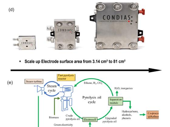
Figure 6. Surface termination (a)-(b), Flow field simulation for electrolyzer (c) Flow electrolyzer from Condias (d), Process loop for electrolyzer integration in existing pyrolysis processing unit (e)
