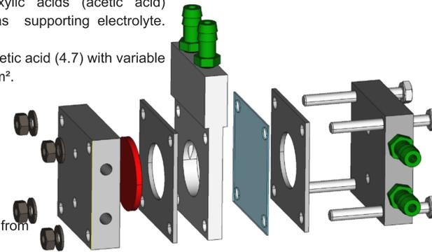
Figure 2. Schematic 3D overview of flow electrolyzer made of stainless steel and designed by Condias.
