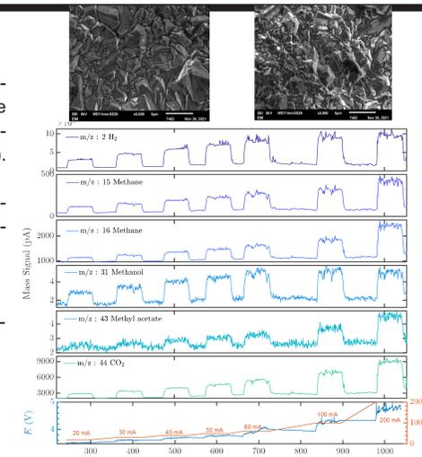
Figure 5. SEM image of BDD after electrochemical decarboxylation (top). In-situ products detections from ECMS for Kolbe/non Kolbe reaction (bottom)
